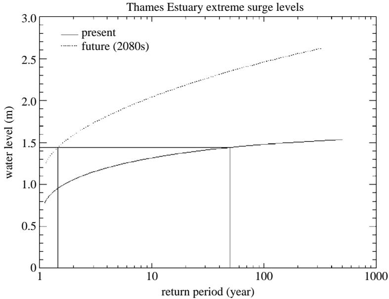
Figure 6. Return period curve for the southern North Sea near the Thames Estuary. Changes in storminess, mean sea-level rise and vertical land movement were included. The future results are for a medium-high scenario following the SRES A2 emissions. The changes are expressed relative to present-day tide.
